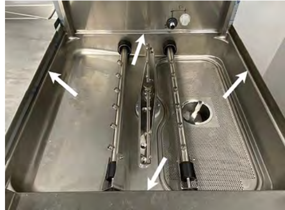
Fig. 29 Wipe along the edges of the tank
