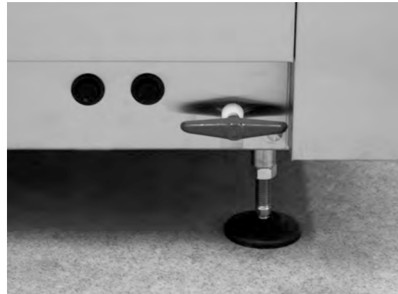
Fig. 28 Access to overheat protectors
