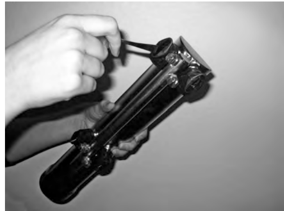
Fig. 24 Cleaning wash nozzles
